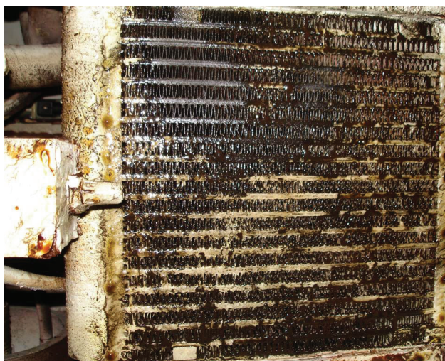
Dirty oil cooler
