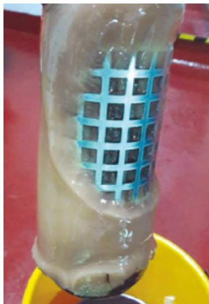
Filter becoming blocked due to build-up of wax. DMA grade bunkered in ARA region - CFPP 5°C
