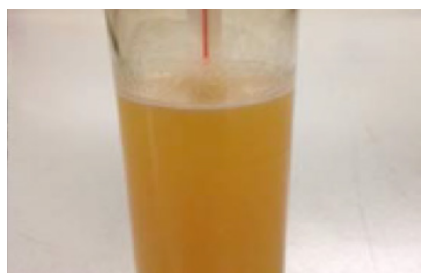
Wax crystals formed at 24°C
