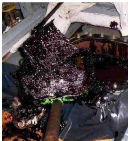
Asphaltene sediment from tank bottom
