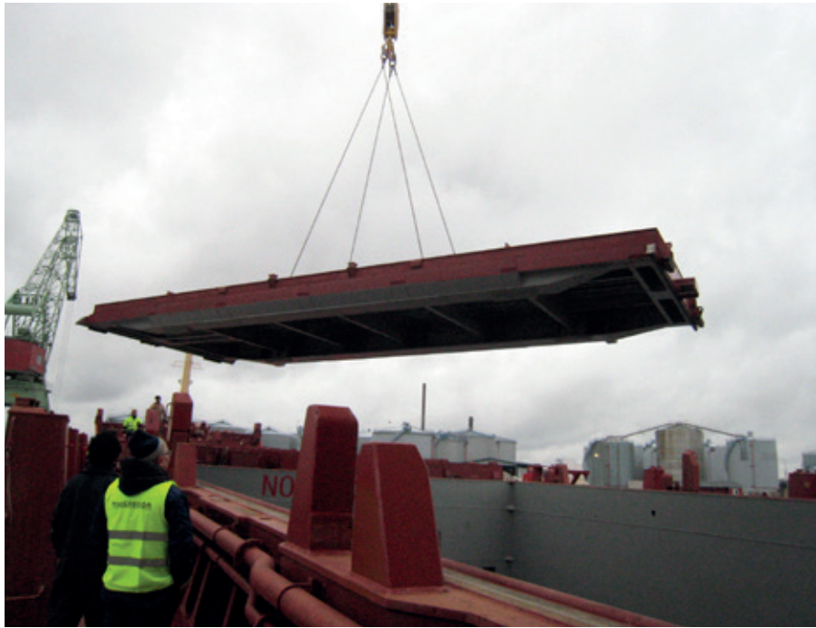
Large pontoon covers for containerships can carry the weight of high stacks of containers.
