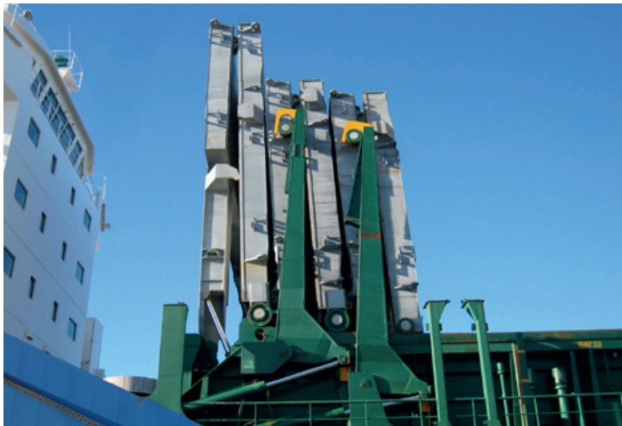
Hydraulic hatch covers became the most popular.
