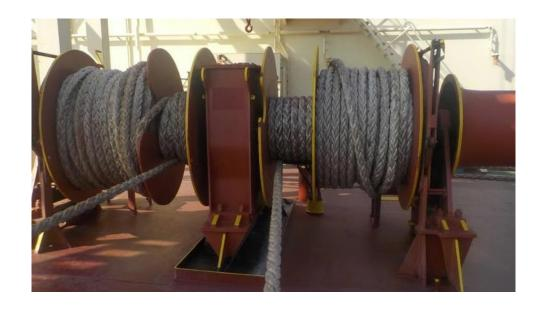
Quick estimate – when drum diameter is 460mm and mooring rope is 64mm, the table shows the reduction of brake holding
